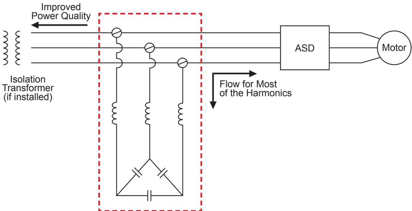
Figure 6 - *Caltrap™* with Line Reactor Harmonic Filter
