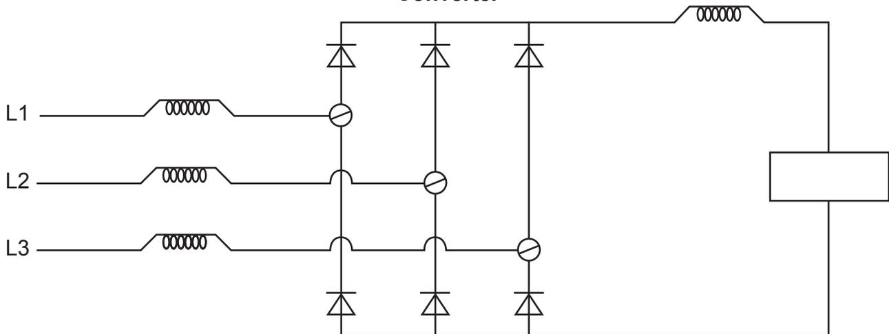
Loads which cause harmonics do so as a steady-state phenomenon. Therefore, if a load is suspected to be non-linear, even an instantaneous reading of the load (while it is operating) can determine if it is harmonic producing.
