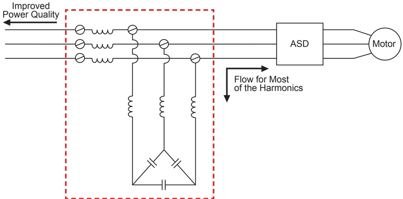
Although the best engineering practice is to trap the harmonics at the source, for economic reasons it may be advantageous to use one trap for several harmonic sources. For example, a machine with several ASDs could be corrected with one trap at the machine control panel. In the same way, several small ASDs fed from one bus duct could have a trap at the beginning of the bus duct, giving the rest of the system better power quality.
